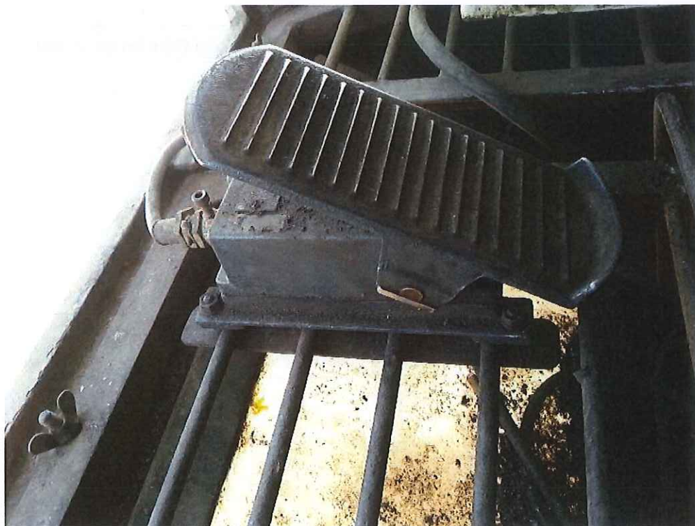
2nd photo: Adjustable braking control pedal E/C 38
